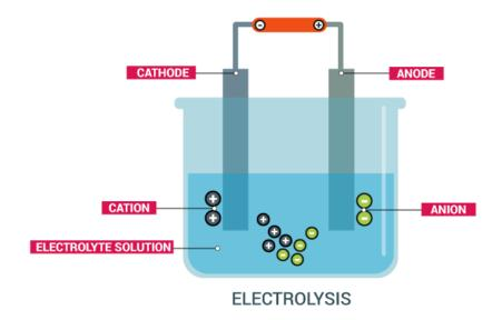
Electrodes are made of graphite or platinum as it is inert (so do not react with the elements)
