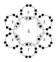
SF<sub>6</sub> has 6 areas of electron density that repel as far as possible around the central Sulphur, hence giving a bond angle of **90**° and a shape to be **Octahedral**.
