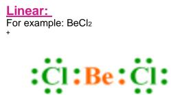
This molecule has 2 areas of electron density around the central 'Be' that will repel <u>as far as</u> <u>possible</u>. This would give a bond angle of **180**° and the shape will be **Linear**.
