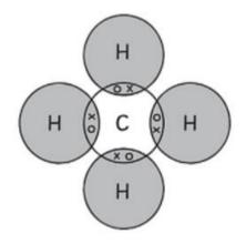
CH<sub>4</sub> has 4 areas of electron density that repel as far as possible around the central Carbon hence giving a bond angle of **109.5**° and shape to be **Tetrahedral**.
