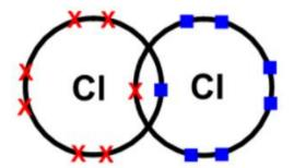
As you can see, one of the electrons in each chlorine atom shares its electron with the other one to produce a full outer shell. This happens because the two electrons are localized between the nuclei of the bonded atoms furthermore, the electrostatic attraction between the negatively charged bonding electrons and the positively charged nuclei holds the atoms together strongly.
