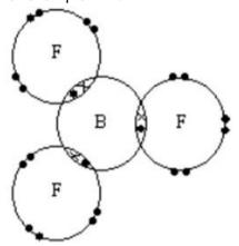
BF<sub>3</sub> has 3 areas of electron density that repel as far as possible around the central Boron, hence giving a bond angle of **120°** and a shape **Trigonal Planar**.
